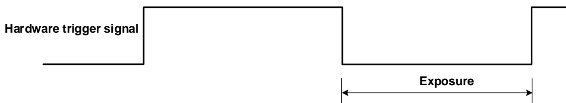
Figure 8-27 The sequence diagram in falling edge trigger of TriggerWidth exposure mode
