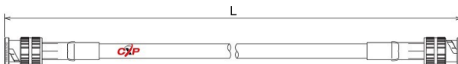
Figure 7-1 the HD-BNC to HD-BNC interface CoaXPress cable
